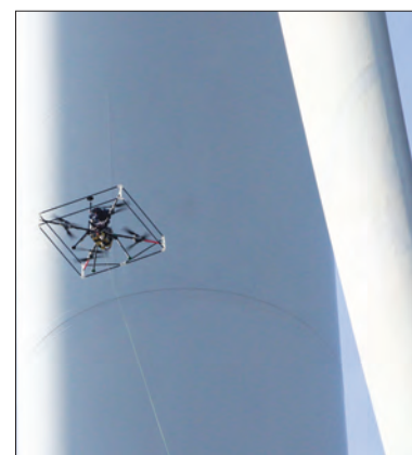
↑ A quadcopter captures images of a wind turbine blade that are then added to an asset management map.
